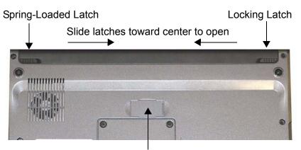
Extended Battery Connector Under Sliding Panel (must be open to install Extended Battery)
